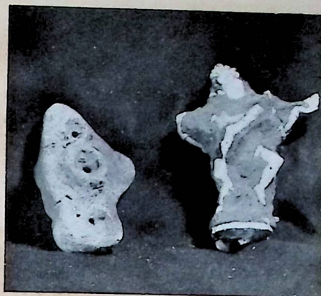
Fig. 3. Half broken mould revealing the image in metal which has replaced the wax one.
