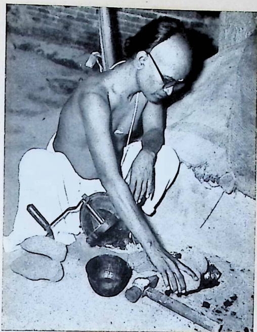
Fig. 2. Breaking up the mould for taking out the cast metal image.
